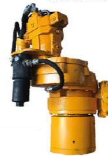
The hydraulic chuck on the rotation unit is synchronized with the rod holder
