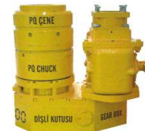
Nitrogen gas spring loaded jaws with hydraulic opening/spring closing function ensuring fail-safe operation.
